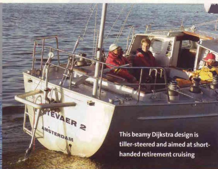
This beamy Dijkstra design is tiller-steered and aimed at short-handed retirement cruising
