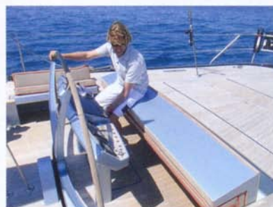
Above: Tulip is the largest project yet for aluminium specialists K&M. From left: owner Melle Boersma steers then shows off the push-button helm seats that rotate to form a flush deck
